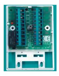
The RC 010-10 has one relay with two separate form C, change over contacts. Each contact has its own screw terminal. The relay operates within the wide voltage range from 9-30V DC. When the relay is energised a red LED indicates to confirm the installation. On the PCB is also a tamper contact that can be used as un opening protection. To simplify the installation there are 10 extra free terminals.
