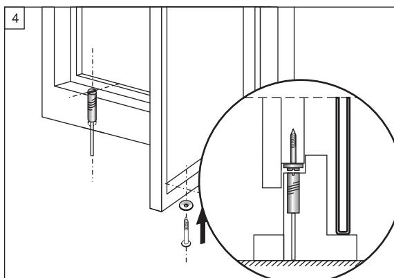
4. Use the screw to fix the magnet into the hole. Correctly mounted the magnet and contact parts must be placed just opposite to each other with a maximum deviation of less than 10 mm. The gap between the two part is up to 15 mm.
