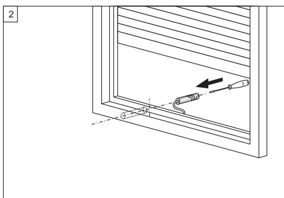
1. Select the place for the contact part at the base of frame.
