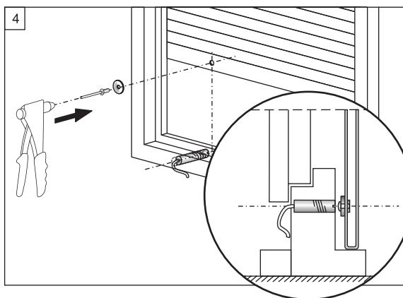
4. Fix the magnet into the roller blind by riveting. Correctly mounted the magnet should be situated on the line of the montage axis of the contact part. Maximum deviation of less than 9 mm.
