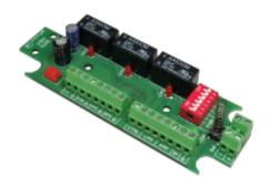
Motor lock alarms are used to control the locking bolt position in a motor lock and ensure that the engine lock is activated or deactivated.
