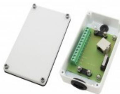
JB RJ45 is a junction box with a RJ45 jack and 12 terminals, 2 of which are intended for the tamper switch. The junction box is intended for alarm and access control systems where a more durable and safe box is needed.
