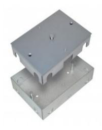
Recess box made of special steel (Magnelis) for mounting of VD 500 in the floor or other hard surfaces. It is designed for mounting and cast into the floor of the museum, vault, safe deposits and gold deposits, and to cope with the pressure of a golden chariot at 5 tons. The box has threaded holes for VD 500 and for mounting a connection box Fatum 28016.03.
