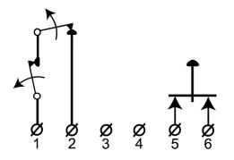
MC 470 is a surface mount high security contact with NC function with 6 screw connections and sabotage contact. The contact is specially designed for use in banks, museums, art galleries, stores, etc.
