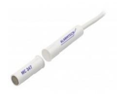
MC 347 is a universal magnetic contact with double NC function that can be used in both alarm and access control systems for monitoring e.g. doors and windows against unauthorized opening. Both the contact and the magnet part are in a water proof (IP 67) plastic housing, which enables easy installation into wood without additional accessories. With our extensive range of installation accessories it is easy to install the contact either recessed or as a surface mount on metal and other materials.
