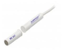
MC 347 is a universal magnetic contact with double NC function that can be used in both alarm and access control systems for monitoring e.g. doors and windows against unauthorized opening. Both the contact and the magnet part are in a water proof (IP 67) plastic housing, which enables easy installation into wood without additional accessories. With our extensive range of installation accessories it is easy to install the contact either recessed or as a surface mount on metal and other materials.
