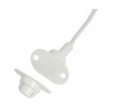
MC 340-S12 is a universal magnetic contact with NC function that can be used in both alarm and access control systems for monitoring e.g. doors and windows against unauthorized opening. This set includes MC 340 and the plastic adapter set MC 300-S12 with a strong magnet enabling recessed installation with screw connection to door and window frames of steel, or in spaces where a larger operation gap is required. Both the contact and the magnet part are in a water proof (IP 67) plastic housing.
