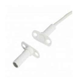
MC 340-S1 is a universal magnetic contact set with NC function that can be used in both alarm and access control systems for monitoring e.g. doors and windows against unauthorized opening. This set includes MC 340 and the small plastic flange set MC 300-S1 for recessed mounting with screw connection in non-magnetic door and window frames. Both the contact and the magnet part are in a water proof (IP 67) plastic housing.
