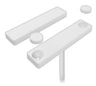
MC 740 is a small and thin magnetic contact with NC function that can be used in both alarm and access control systems for monitoring e.g. doors and windows against unauthorized opening. Both the contact and the magnet part are in a water proof (IP 67) plastic housing. The small and thin format makes it especially easy to install in limited spaces, e.g. on shutters and drawers.
