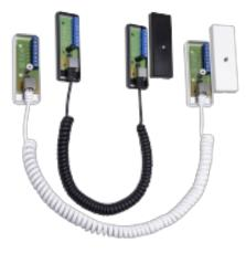
DL 6A is a door loop that consists of a 6-pole flexible spiral cable with RJ12 modular connector at both ends and two junction boxes (JB 103-6) with modular connector connection and 8 screw connections of which 2 are for the opening contact.
