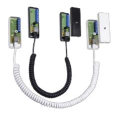
DL 6A is a door loop that consists of a 6-pole flexible spiral cable with RJ12 modular connector at both ends and two junction boxes (JB 103-6) with modular connector connection and 8 screw connections of which 2 are for the opening contact.
