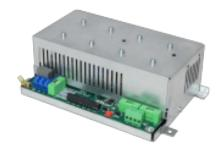
Power supply unit as a module for DIN-rail mounting with ViP (Voltage in Parallel) function, 12 VDC 3,5 A.
