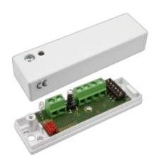
CD 470 offers reliable monitoring against attacks with mechanical tools. The CD 470 is a chock- and vibration sensor with 3 separate detection channels: an integration channel / saw channel for weak signals with long duration, a counting channel that senses strong impact on the monitored surface and an explosion channel which senses very strong signals from e.g. an explosion.
