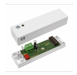
CD 475 offers reliable monitoring against attacks with mechanical tools. The CD 475 is a chock- and vibration sensor with 3 separate detection channels: an integration channel / saw channel for weak signals with long duration, a counting channel that senses strong impact on the monitored surface and an explosion channel which senses very strong signals from e.g. an explosion.
