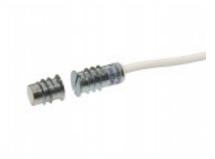
MC 250 is a universal magnetic contact in small format with NC function that can be used in both alarm and access control systems for monitoring e.g. doors and windows against unauthorized opening. Both the contact and the magnet part are made of Al-alloy and formed in the shape of a threaded screw, which enables easy installation into wood or plastic. With our extensive range of installation accessories it is easy to install the contact in different kinds of doors and windows.
