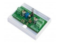
FATUM mini DC-DC converter is an easy-to use 32 V, 2 A synchronous step-down regulator.
