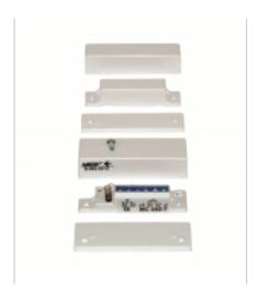
MC 440-T is a surface mount magnetic contact with NC function and with 6 screw connections. It can be used in both in alarm and access control systems for monitoring e.g. doors and windows against unauthorised opening.
