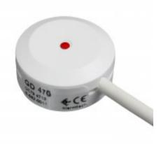
The passive glass break detector GD 470 is suitable for float, tempered, laminated & reinforced glass. The GD 470 is glued to the glass surface and will detect various attacks (including cutting tools) on the glass surface.
