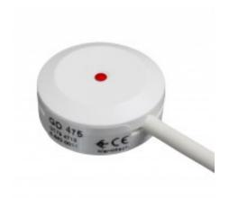
The passive glass break detector, GD475, is certified to EN Grade 3 and is suitable for float, tempered, laminated & reinforced glass. The GD475 is glued to the glass surface and will detect var-ious attacks (including cutting tools) on the glass surface. The detector requires an interface unit IU400, which senses the changes in the current characteristics of the detectors and provides alarm and fault outputs.
