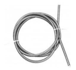
Flexible and durable armoured flexi-tube cable protection in stainless steel. Suitable for protection of cables in exposed environments. Plastic conduit in each end of the steel tubing protect cables from wear or breakage. Outside diameter of 14.0 mm and inner diameter of 10.5 mm. Maximum cable diameter of 8.8 mm. The armoured flexi-tube cable protection is compatible with the DL H14 mounting plate/end caps and corresponds to the metal tubing in the DL 14 cable loop.
