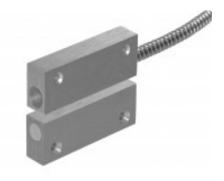
The MC 240-S45 set is intended for exposed environments where a more durable magnetic contact is needed, such as doors, gates, etc. The set consists of MC 240-C contact with a NC contact function installed in MC 200-4 Al housing and an extra strong magnet in MC 200-5 Al housing, which allows for a wide opening gap.
