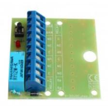
The RC 010 is a relay card with a dual (2x) alternating (NC / NO) function. Connection is provided via screw terminal with wire protection. Active relay is indicated by LED. The card also has an anti-tamper switch to protect against unauthorised opening if the card is installed, for example, in a JB 200 box.
