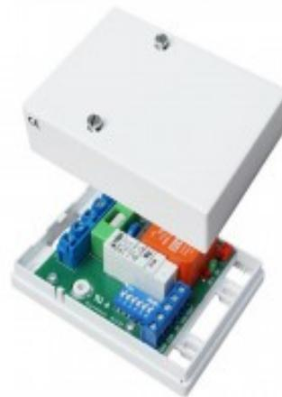
RC 230 enables control of a high voltage load up to 2000 VA with a magnetic contact or low voltage detector. It has a built-in programmable timer function for ON or OFF control. The time is programmed with a DIP-switch, from 0 s to 16 hours. The high voltage relay has a changeover function that can switch 250 V AC max 8 A. The relay circuit is protected by a 10 A fuse.
