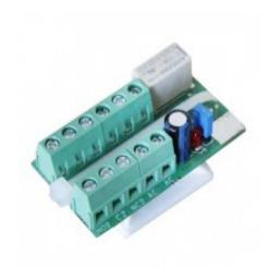
The RC 4 is a compact and universal relay card for AC or DC supply with dual alternating (NC / NO) relay function 2A. Connection is provided via screw terminal with self-lifting clamp.
