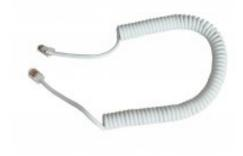
Der DL S8 coiled cord door loop with 8 leads and RJ-45 connector in both ends. The door loop is designed for sliding doors, gates, overhead doors where an extendable cable is needed. DL S8 are a made of PUR material (cable track cables are particularly for continuously flexible use), this makes the door loop more elastic and resistant against sunlight, chemicals, etc. The door loop is available in two sizes, 100 cm and 250 cm (extended length). DL S8 can be used together with JB RJ45.
