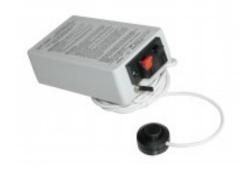
Hand-held test unit for glass break and vibration detectors. Generates two types of test signals, one for GD 300/GD 400 and one for VD 400 detectors. Also contains a 12V output for test of GD 300 and 400 series before mounting.
