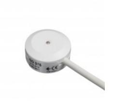
The GD 375 is a passive glass break detector with transistor output that is connected to a control panel via an IU 300 interface unit. It is designed to protect laminated glass in application areas as shop-windows, glass sliding doors, standard windows and other vulnerable glass surfaces in public areas and private homes.
