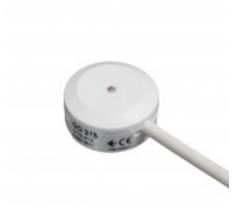
GD 375 is a passive glass break detector glued on to the glass surface. Together with interface IU 300 it forms a Grade 2 security system according to EN 50131-2-7-2 to detect an attack against float glass through smashing with blunt force or cutting or drilling with diamond tools. Application areas are shop-windows, glass sliding doors, standard windows and other vulnerable glass surfaces in public areas and private homes.
