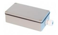
Metal housing with integrated heating element for the CD 400 and VD 400 when the detectors are mounted in cold and damp areas. The housing is supplied with anchor bolts, which ensure a wide detection area and an 150-ohm resistor that functions as internal heating. The current consumption of the resitor is 80mA / 1W at 12V AC / DC and 160mA / 4W at 24V AC / DC, in both cases the effect is enough to prevent from a moisture inside the housing.
