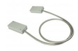
The VD 500 seismic detector provides reliable detection and high immunity to false alarms when mounted on steel or concrete objects such as firearm cabinets, payment terminals, ATMs, safes, concrete walls etc. It detects intrusion attempts with explosives and mechanical tools such as diamond drills, cutting discs, grinding and thermal tools.
