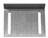
L-shaped installation bracket of aluminium, with hole patterns suitable for most of the MC 200 and MC 300 accessories as well as the MC 400 series. Manufactured of 2 mm anodised aluminium.
